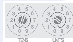
Figure 10: Decade address switches address 03 selected
