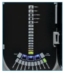
FAAST<sup>TM</sup> User Interface Display The User Interface consists of 5 Alarm levels – Alert, Action 1, Action 2, Fire 1, and Fire 2, 10 Particulate levels, 10 Bi-colour Flow and Fault graph.
