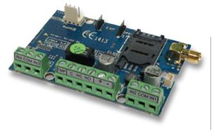
GSM/GPRS communicator with alarm center features. The device can be expanded with a range of accessories so it has a wide application range.
