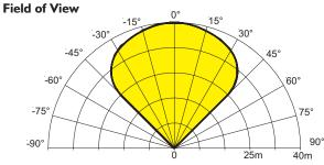
To meet the requirements of EN54:10 dause 5.4, where the ratio of the response points Dmax:Dmin should not exceed 1.41, the horizontal and vertical viewing angles  $\alpha$ max should not exceed  $\pm 30^{\circ}$ .
