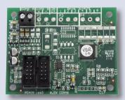
The Esento Marine VDR (Voyage Data Recorder) output card is a plug in communications card for the Haes Esento Marine range of fire alarm control panels
